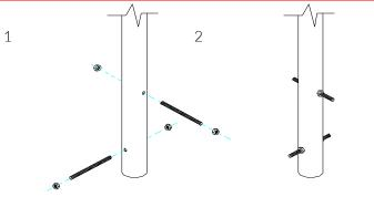
Insert M10x 150 Threaded bar into pre drilled holes in Ground Fixing Post
