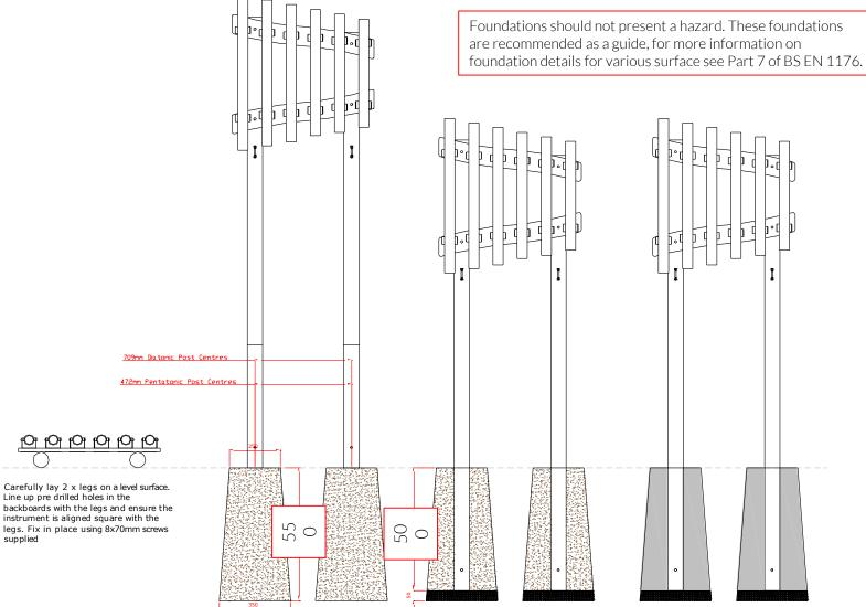
Excavate 2 holes with a 250mm diameter tapering down to 350mm diameter and minium 650mm depth
